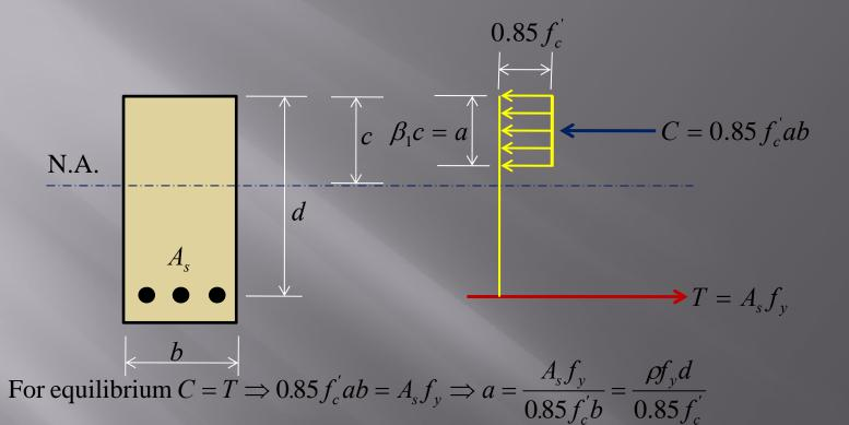
where  $\rho = \frac{A_s}{bd}$  = tensile steel ratio. Because the reinforcing steel is limited to an amount that it will yield well before the concrete reaches its ultimate strength.
