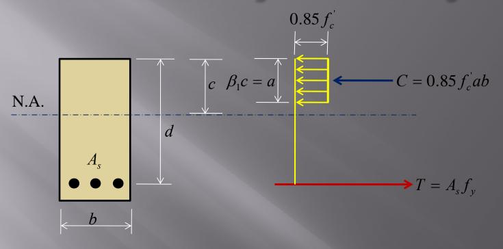
Theoretical or nominal flexural strength/resistance (or resisting moment) of a section is denoted by  $M_n$ . The design/usable flexural strength/resistance=
